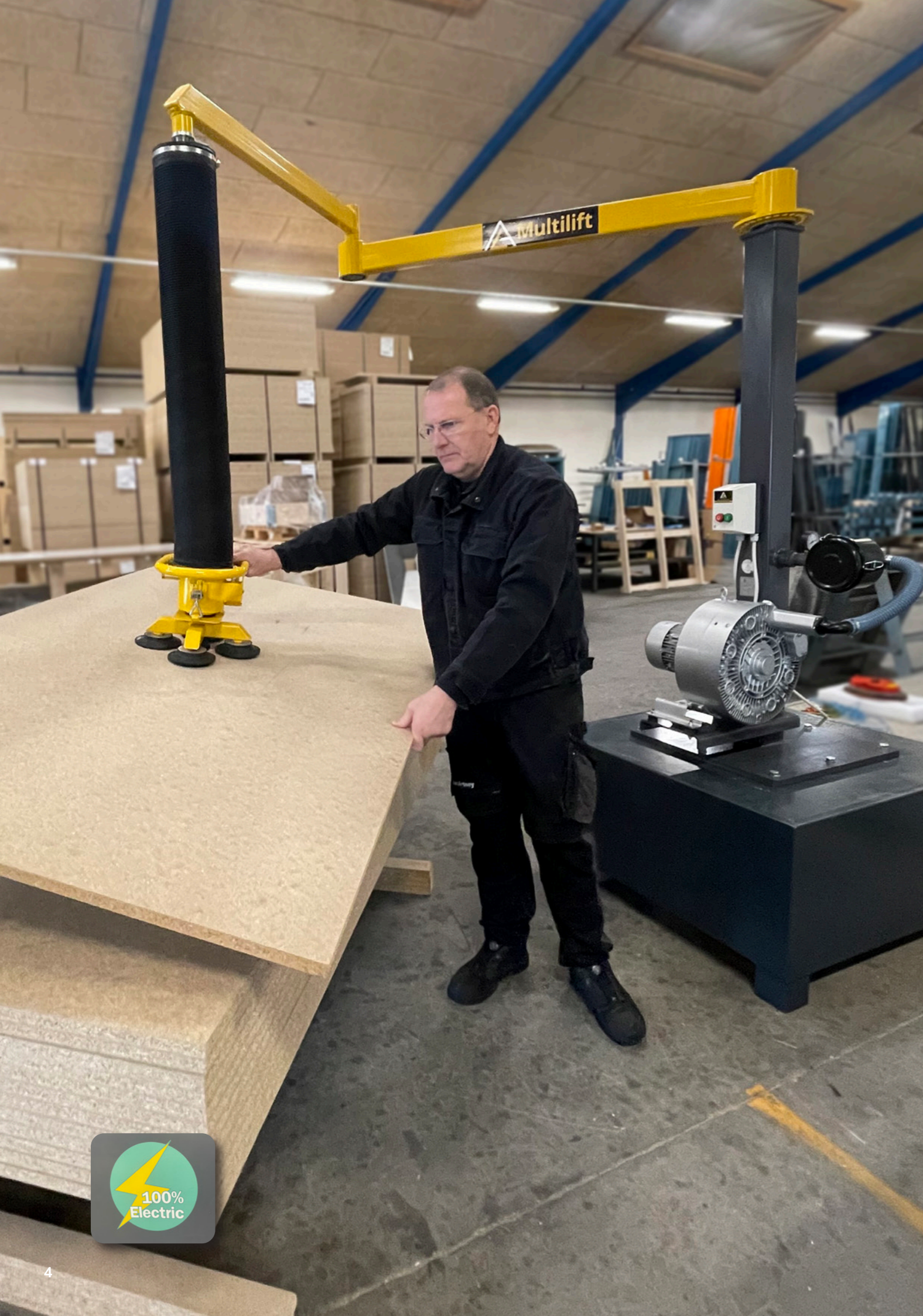
The two-part arm with maintenance-free ball bearings in the bearing housing makes it easy to set in motion.
