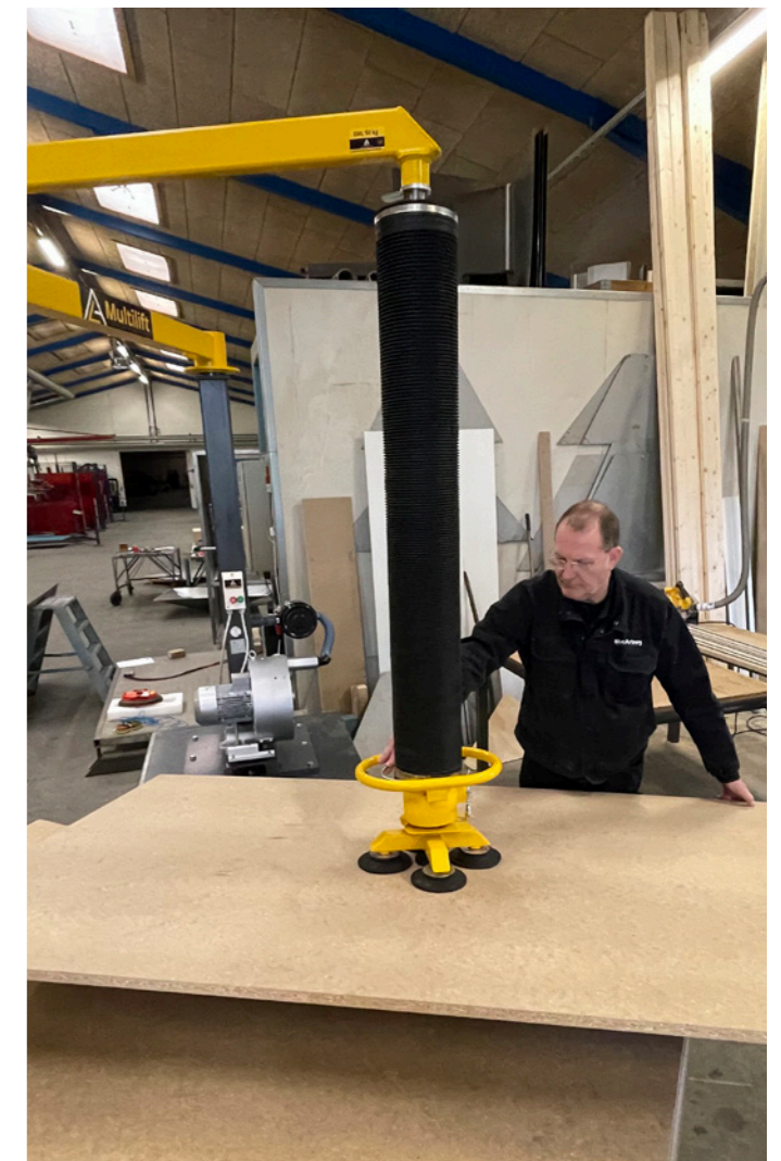
Vacuum passes inside the main seats, through the bearing housing and out into the arm to the vacuum lift hose.
