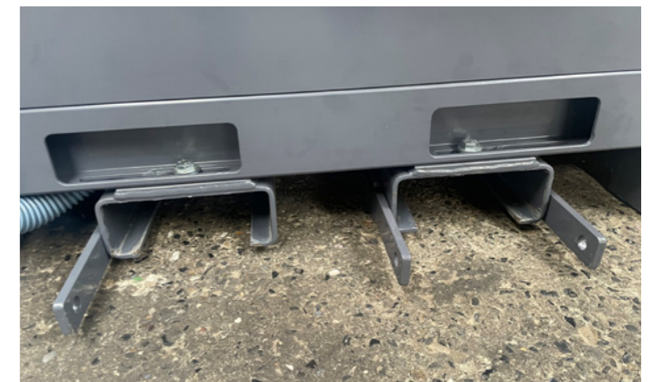
Changeable fork pockets inner dimensions - 190 mm wide, 70 mm high. Each fork can be adjusted by 170 mm
