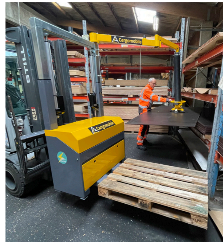
The front panel can be removed so you can change the battery case in a few minutes
