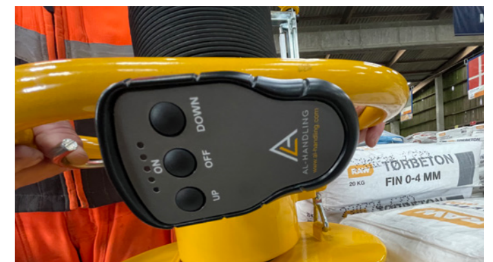
Start/stop of the vacuum pump and lifting/lowering the mast is done remotely
